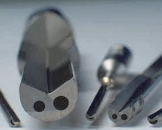
The trend towards multi-station machining has resulted in single-lip drills being used increasingly on conventional machine tools, for example on machining centres. With its combination of precision and superior drilling performance, the single-lip drill is also used for short and intricate holes.
