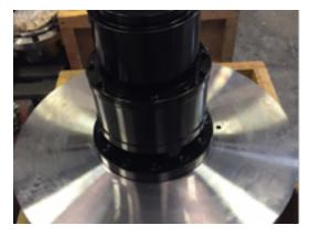
Gear coupling with brake disc.
