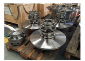
Disc pack configuration with brake disc.
