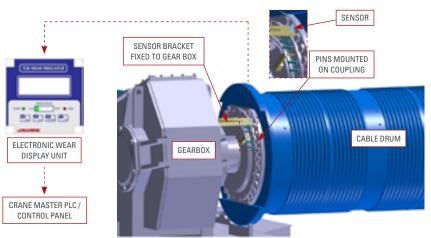
Fig. nº. 16. Electronic wear indicator working layout
