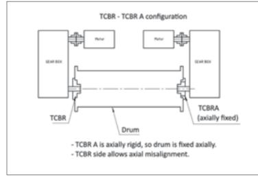
Barrel coupling TCBRA is not designed to support axial load. For each size, there is a maximum value that the coupling can withstand:
