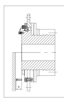
Fig. n.° 13. Distance necessary for screw removal.
