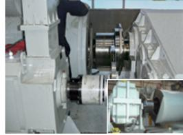
Barrel and gear coupling with brake disc.
