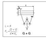
Fig. n.° 10. Hoist, 2 sheaves. Single line to drum.
