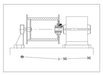
Fig. n.º 2. Fig. n.º 3. Rigid mounting of gearbox-drum connection. Support at three points. Mounting with barrel coupling.
